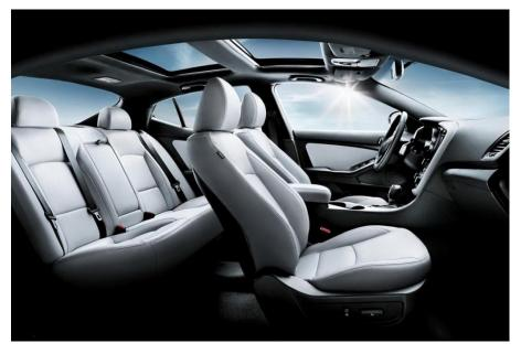
14. Panoramic sunroofs present manufacturing, design, and safety challenges for manufacturers because the large plates of glass take up much of the surface area of the vehicle's roof.
